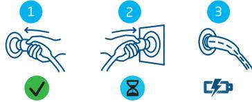
Figure 4.3: Starting the charging process without charge card. Symbols shown on user interface
