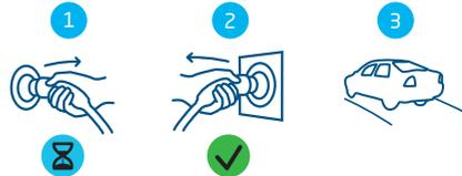
Figure 4.4: Stopping the charging process without charge card. Symbols shown on user interface
