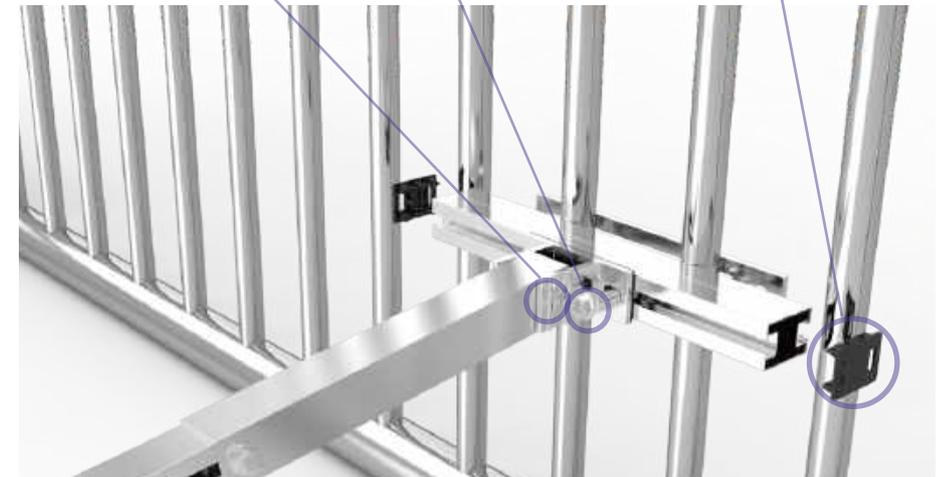
4.15 L foot installation and connection: The L foot is locked on the other side of the panel frame with bolts, and then connected with the telescopic rod with bolts;
