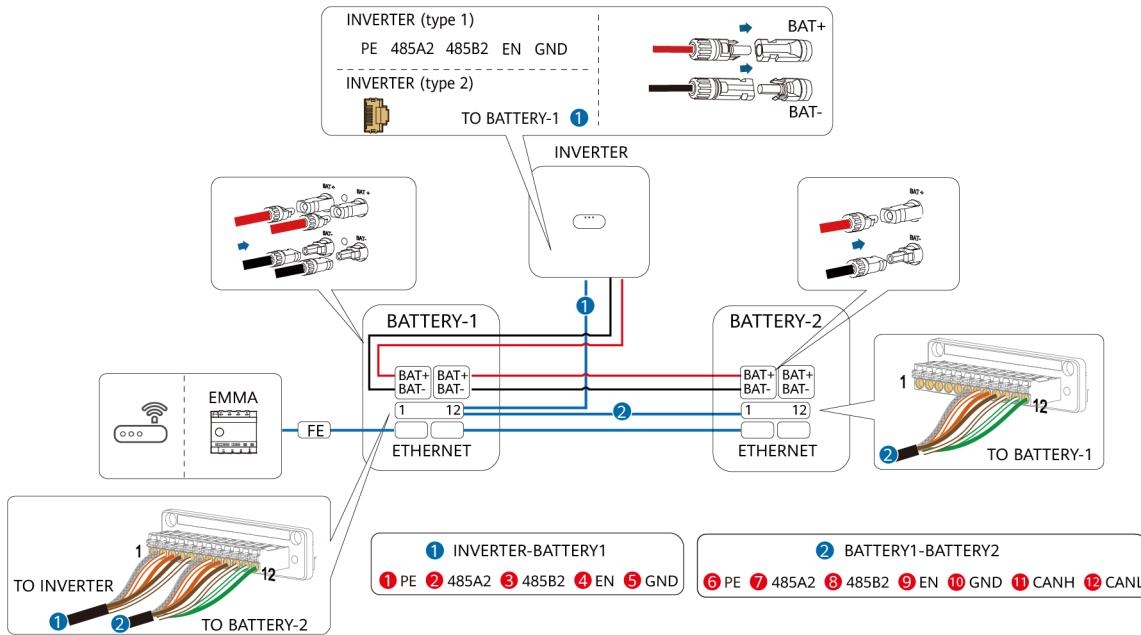
**EN** For details about how to connect parallel cables, see the user manual.
