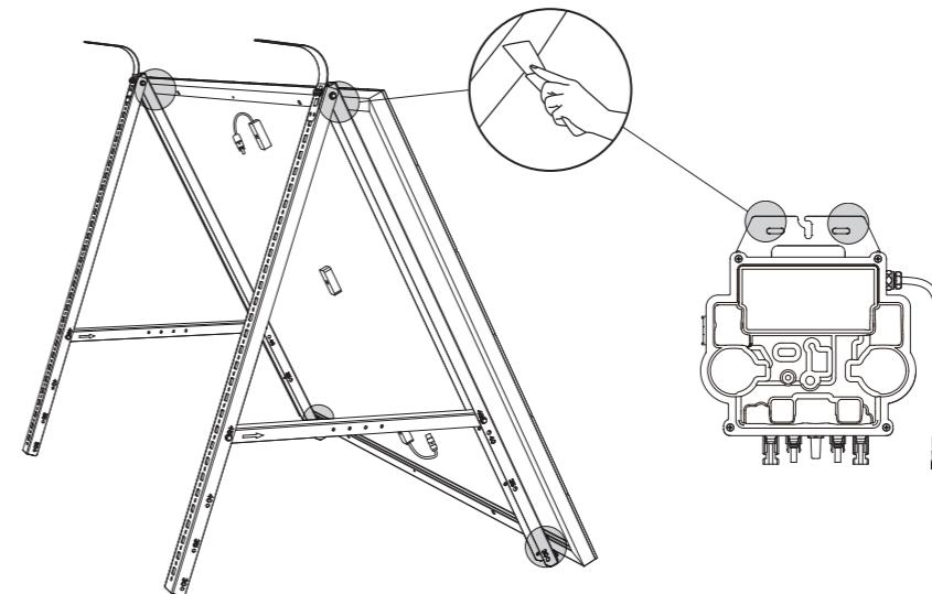
The solar system does not need to be struck by lightning to cause damage. A strike nearby often induces voltage spikes in the electrical grid that can damage equipment. The microinverter has surge protection, but if the surge has sufficient energy, the protection built into the microinverter can be exceeded—causing damage to the equipment.
